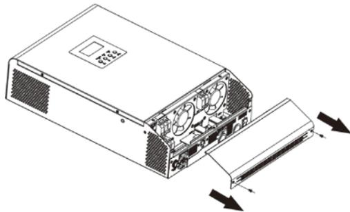
**Step 2:** Remove communication board by unscrewing two screws as below chart.
