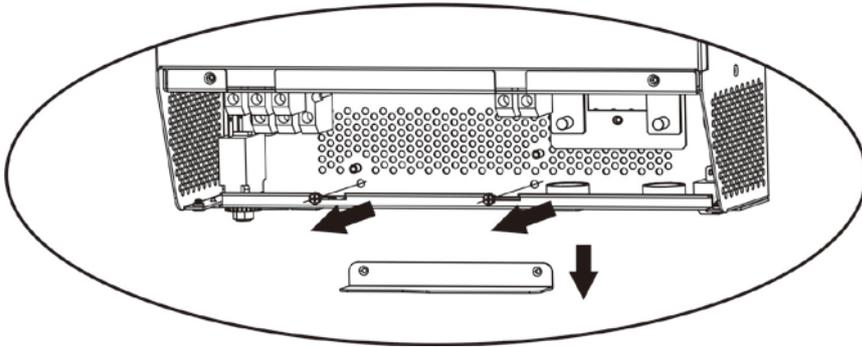
**Step 5:** Install new parallel board with 2 screws tightly.
