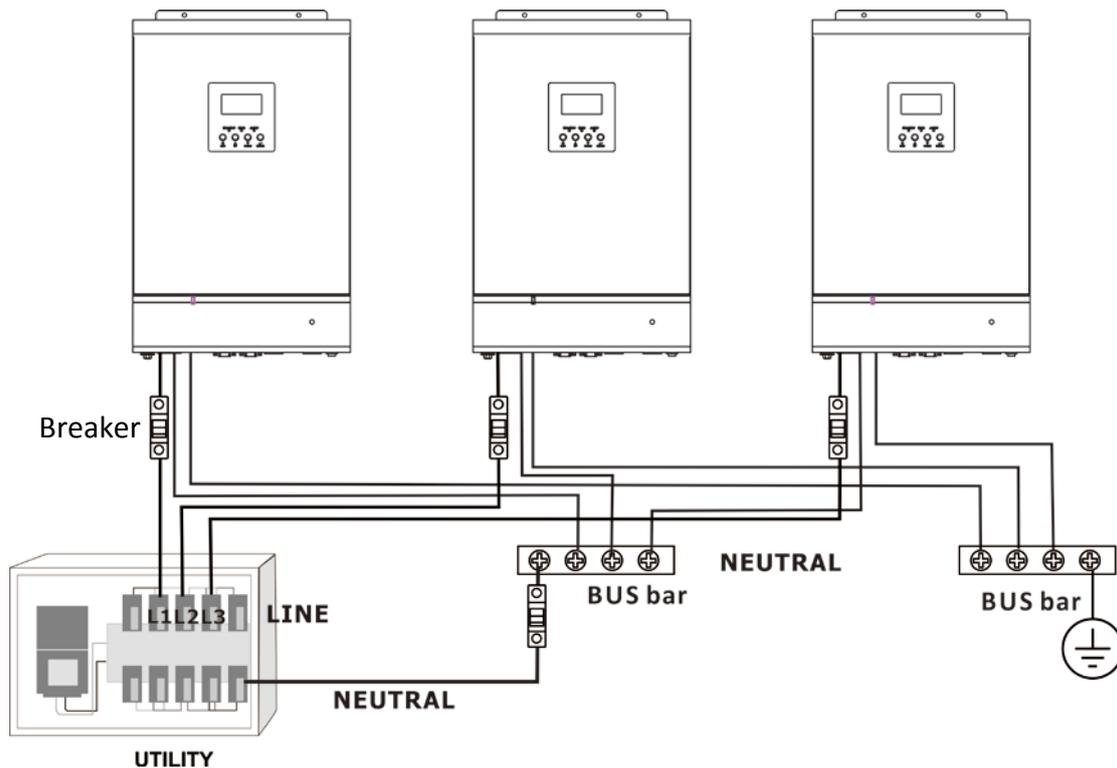
**WARNING:** Only Line wires can be connected breaker. It's not allowed to add breaker into Neutral wires between inverter and the BUS bar. All Neutral wires are connected to the BUS bar directly, and you can add a breaker between the utility and the bus bar in the distributor.
