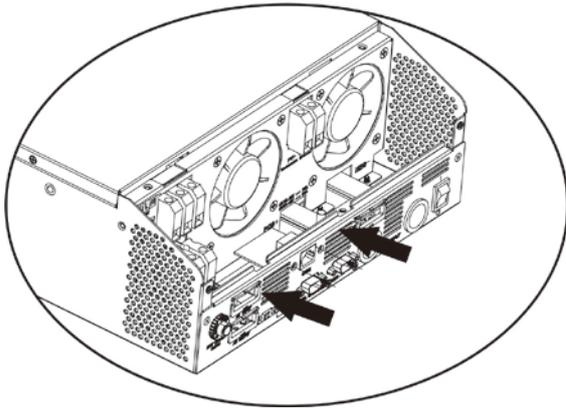
**Step 8:** Put wire cover back to the unit. Now the inverter is providing parallel operation function.
