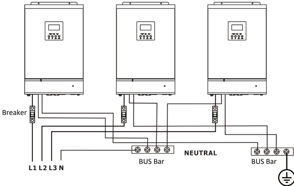
**WARNING:** Only Line wires can be connected breaker. It's not allowed to add breaker into Neutral wires. All Neutral wires are connected to the BUS bar directly.
