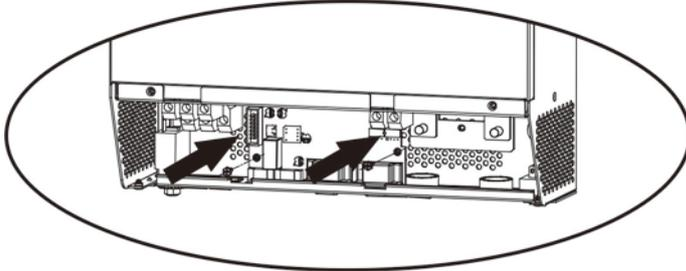
**Step 6:** Re-connect 2-pin and 14-pin to original position.
