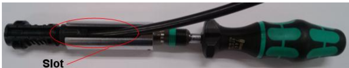
Figure 9 Tightening of the cable screw joint nut (initial tightening torque is 1.8 \pm 0.1 \text{ Nm} )
