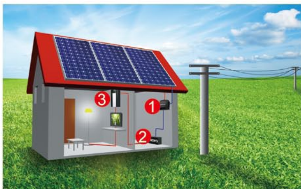
① MPPT ② Battery ③ Inverter
